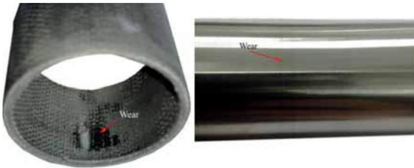
Figure 4. Composite slide bearing and shaft wear
